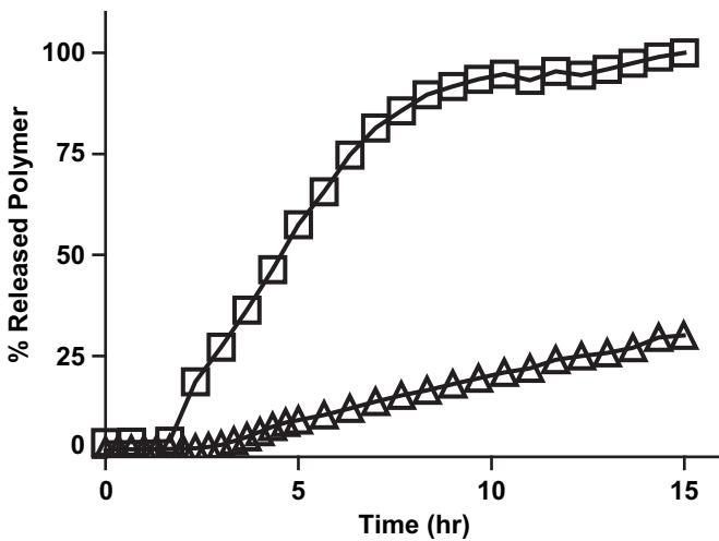
**Fig. 4.** Leaching of polymer from electrospun fibers. A: Time-course of polymer **4** leaching from CF-**4** fibers empty squares no UV, empty triangles UV irradiated fibers.
