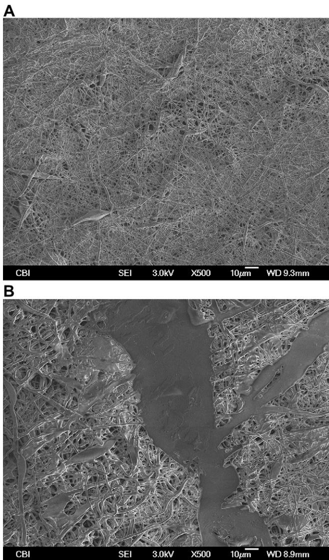
**Fig. 3.** SEM pictures of electrospun CF with the soluble polymer **4** before (A), and after (B), UV irradiation at 330–350 nm for 5 min.
